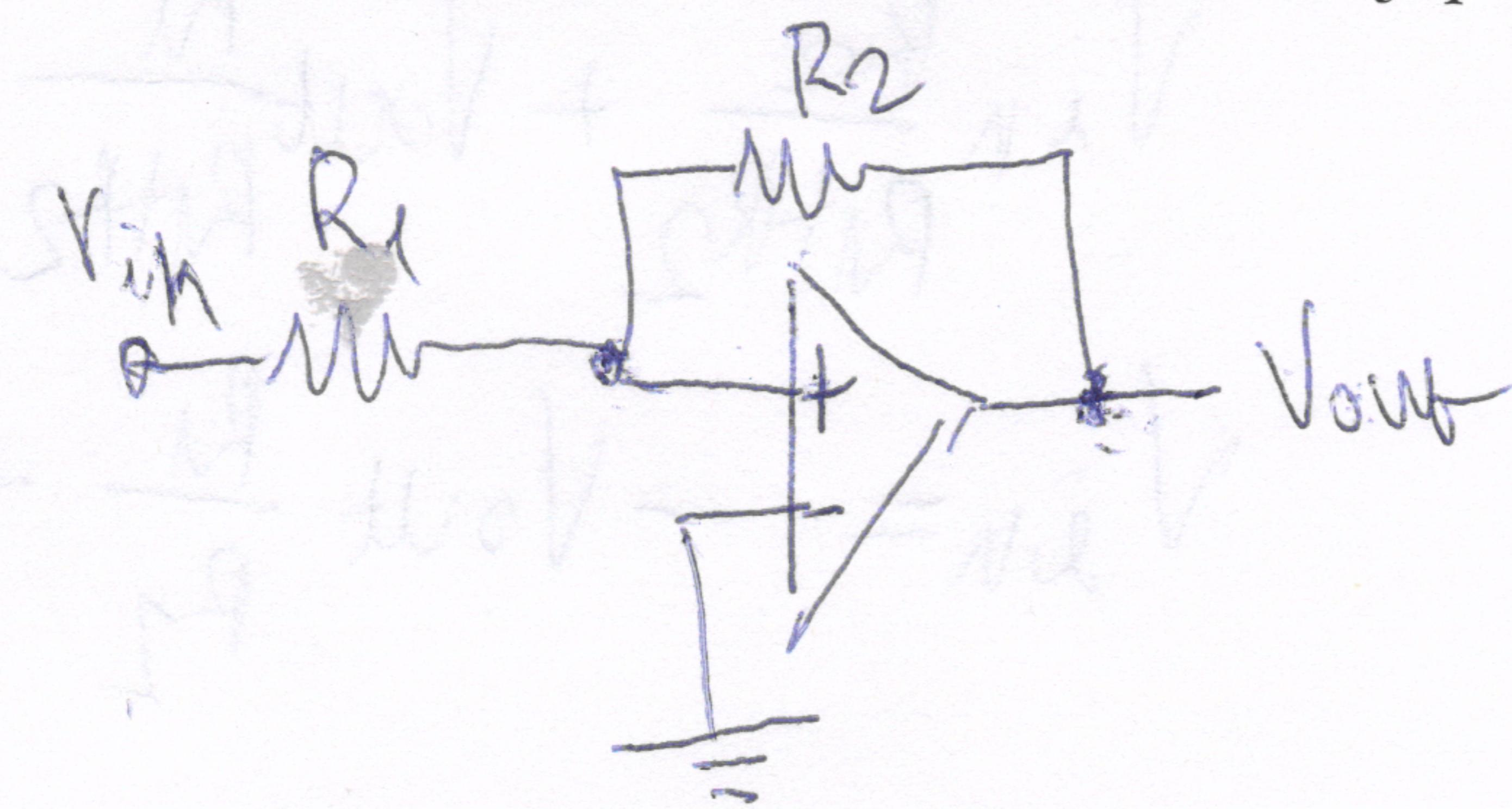
$$V^+ = \frac{R_2}{R_1 + R_2} \cdot V_{in} + \frac{R_1}{R_1 + R_2} \cdot V_{out}$$
