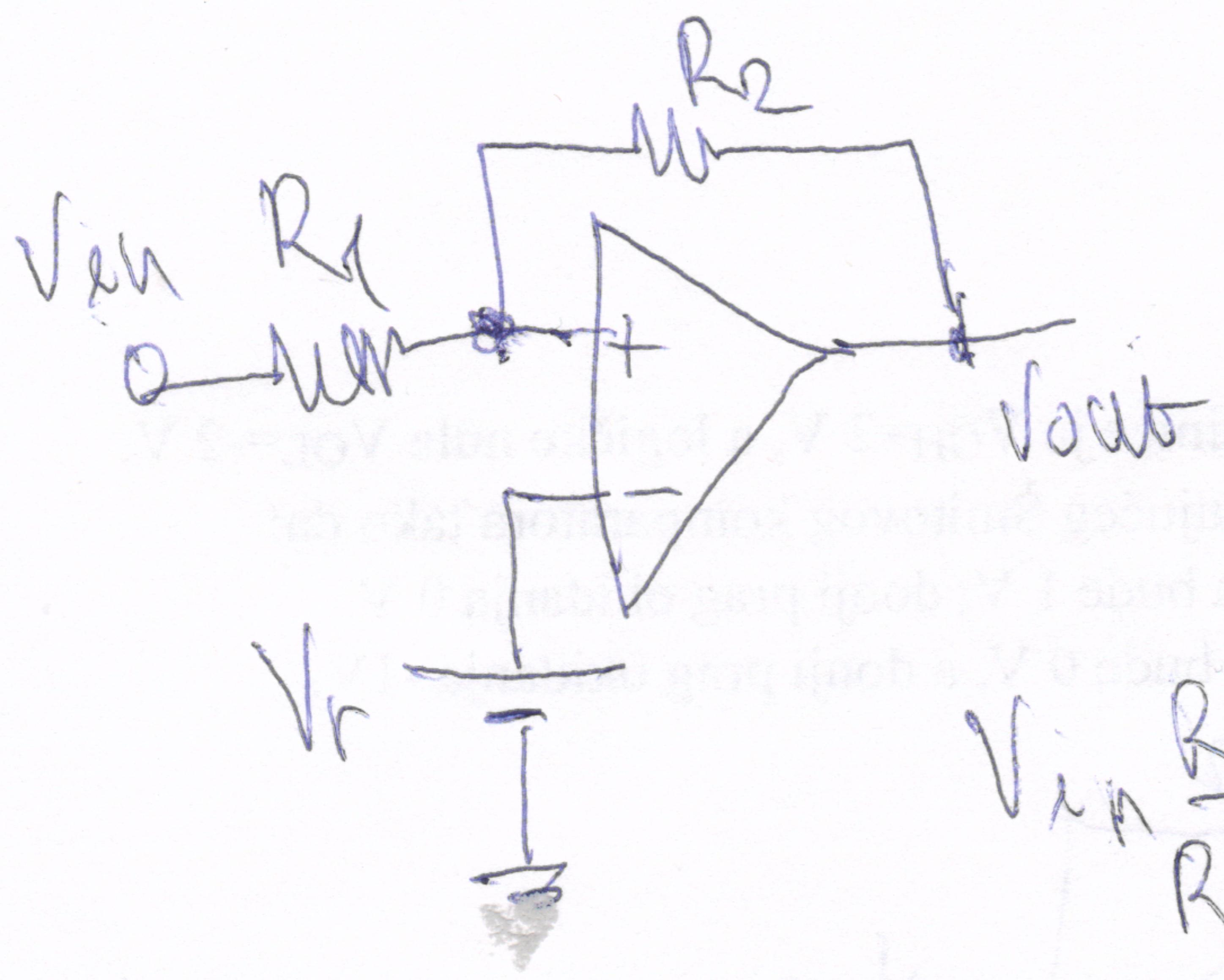
$$V_{in} \frac{R_2}{R_1 + R_2} + V_{out} \frac{R_1}{R_1 + R_2} = V_r$$
