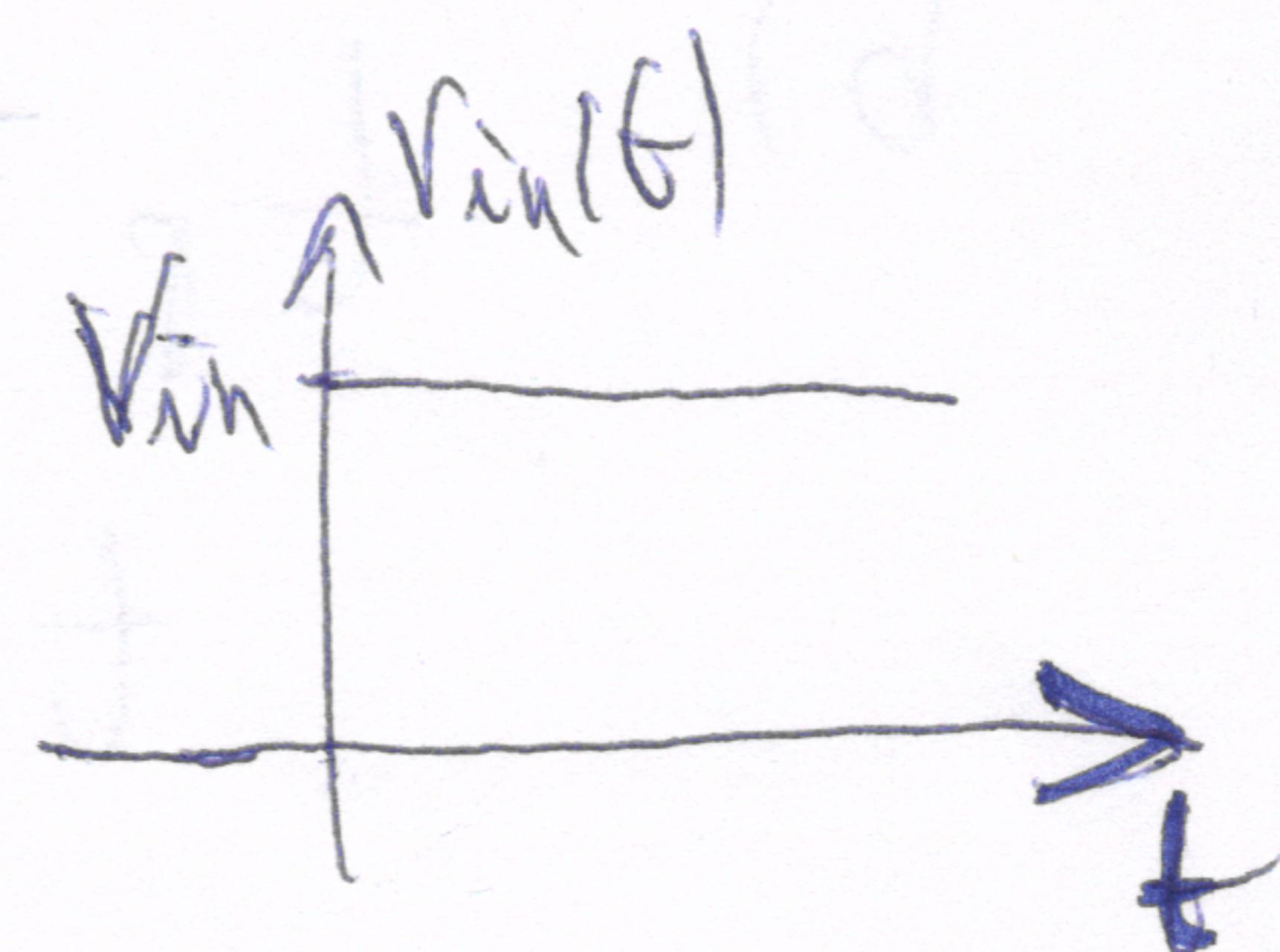
$$V_{in}(s) = \frac{V_{in}}{s}$$
