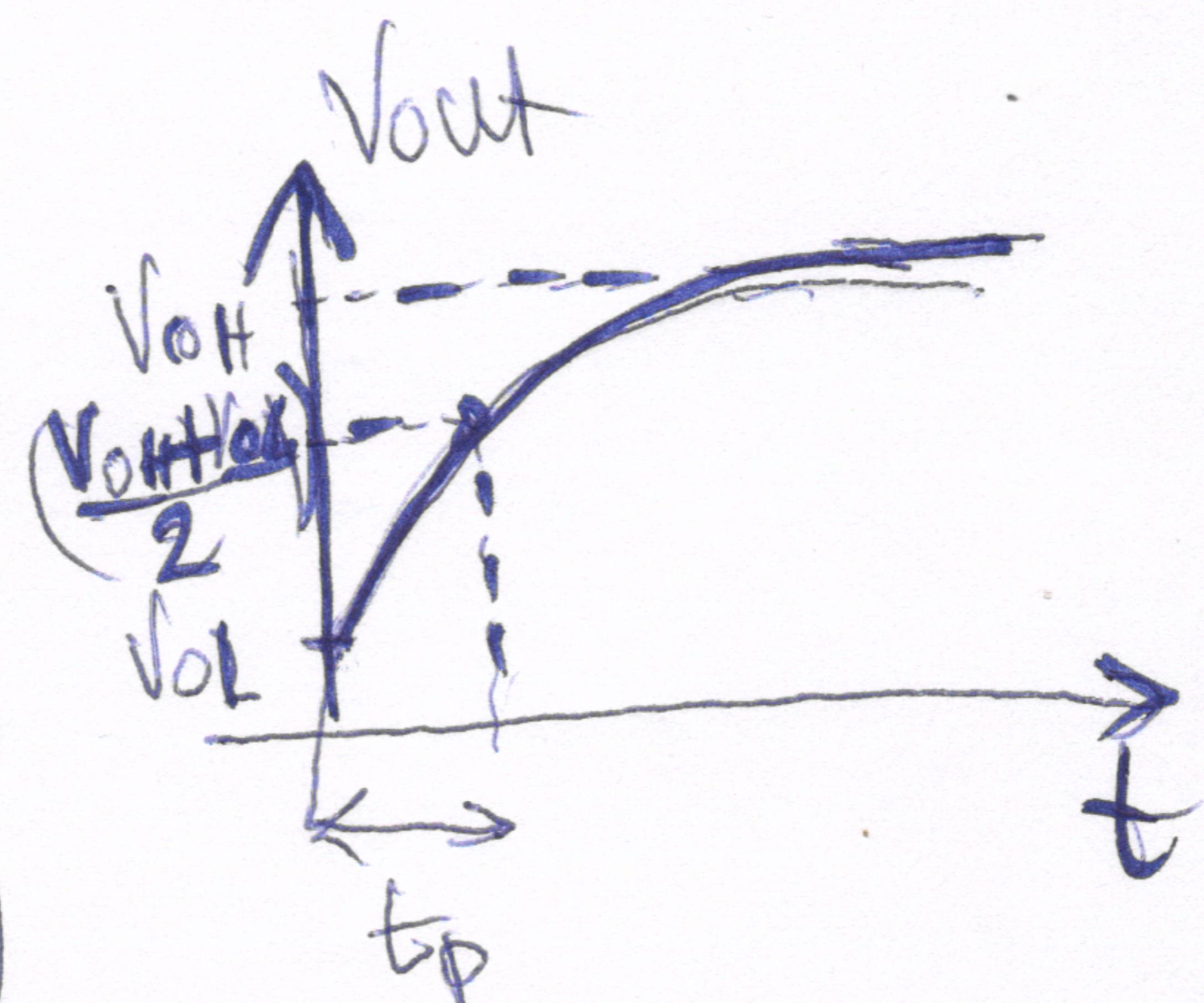
$$A_0 \cdot V_{in} \left( 1 - e^{-\frac{t_p}{T_p}} \right) = \frac{V_{H+L}}{2}$$
